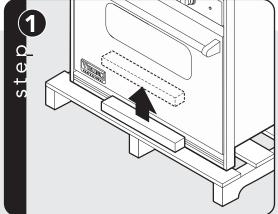
Remove wooden brace on front of pallet.
